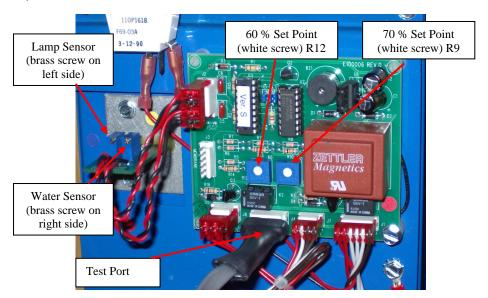
Use the Adapter cable to plug into the port marked 'TEST'. This will cause the four values to appear on the Hallett Diagnostic Tool. If there are no values on the display, disconnect the cable at the Hallett Diagnostic Tool end and then reconnect it. In some cases, plugging in the Hallett Diagnostic Tool may cause the UV unit to beep and cycle the solenoid valve off & on. This is momentarily caused by the start up of the display but will return to normal.
